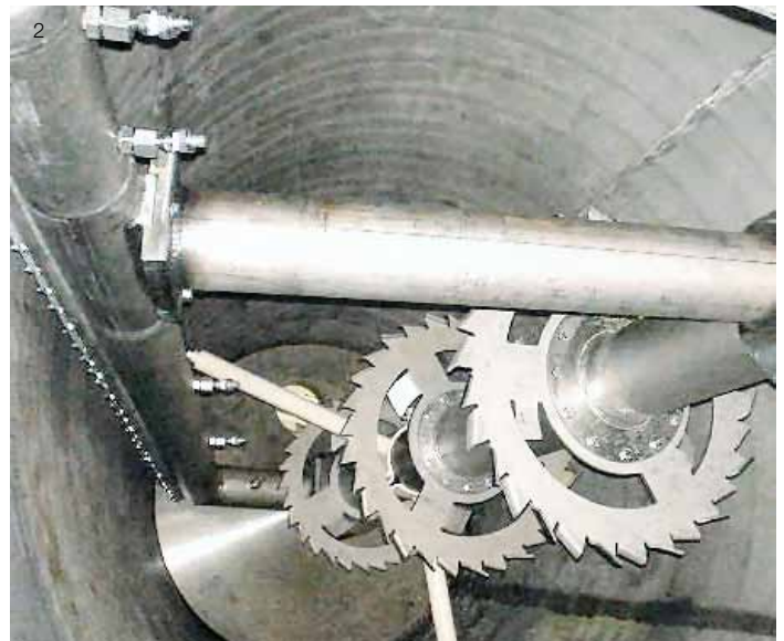
1 | Inside view of the Delicel™ with dispersion toothed turbines 2 | Inside view of the CIP Delicel™ with cleaning nozzles on peripheral mixing unit
